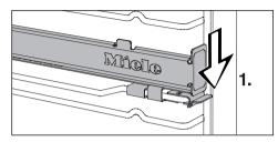
Push down on the tab at the front of the FlexiClip runner (1.).
